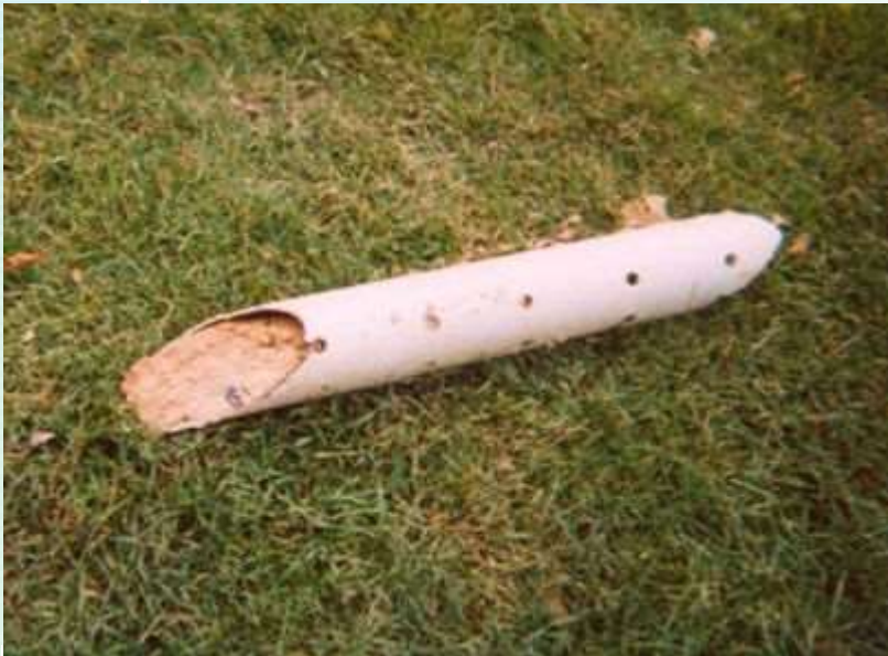
Slotted pipe often block.
