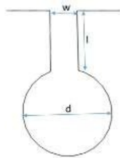
Appendix Fig.1-1 Schematic diagram of capiphon hole
