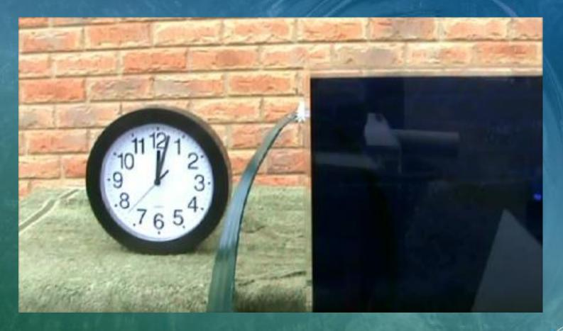
The tank contains dyed water. Water begins to flow through the belt almost immediately even as the tank continues to fill.
