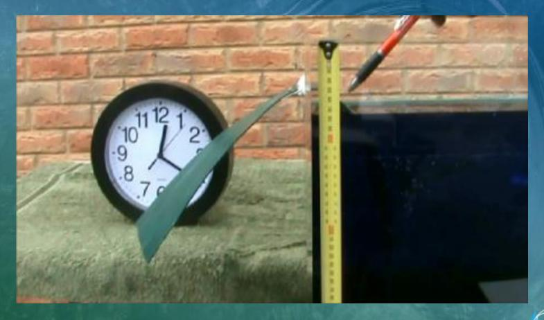
After about 20 minutes the water level in the tank has dropped to about -35mm. The belt is still dripping but only slowly.
